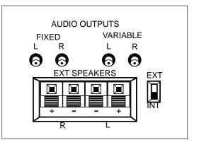
The FIXED/VARIABLE OUT jacks on the back panel provide a fixed or variable audio signal. When connected to "variable", they are ideal for use with an audio amplifier that does not have its own remote volume control. When connected to "fixed," the output volume stays the same no matter how the volume changes on the TV.
