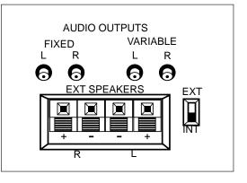
When connecting the speaker wire, make sure you connect the positive (+) terminal on the TV to the positive (+) terminal on the speaker. One side of the speaker wire is usually marked with a white stripe to help you match the terminals correctly. If the (+) and
