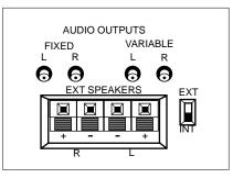
To turn the TV's internal speakers on and off, press MENU on the remote control and choose *Audio*. Then choose *Speakers* from the menu.
