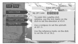
5. Record the elevation, azimuth, and tilt (oval satellite dish only) numbers below.
