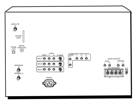
**SATELLITE IN** Use to connect the satellite dish antenna to the TV using an RG6 cable.
