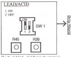
12 volt -14.5 high - 13.3 float (volts at battery)
