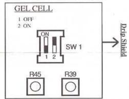
12volt 14.1 high - 13.8 float(volts at battery)
